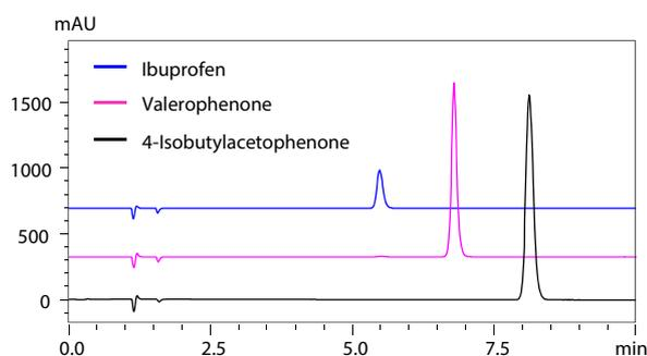
**Fig. 5 Chromatograms of Fractions Obtained by UFPLC**
