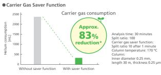
Comparison of helium carrier gas consumption per analysis with and without the carrier gas saver function
