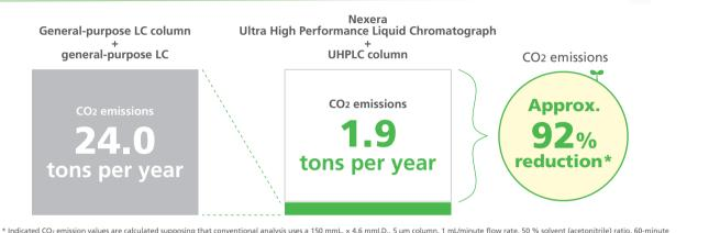
analysis time, 10 analyses per day, with 10 LC instruments operating 240 days per year, while UHPLC analysis uses a 50 mml. x 2.0 mml.D., 2.2/2.6 µm column, 0.5 mL/minute flow rate, 8-minute analysis time. However, these differ due to operating environments and analysis details. In addition, CO2 emission values are calculated from the power consumption using a conversion coefficient.
