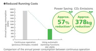
of a previous Shimadzu model and the GC-2025 using automatic start/stop functions.
